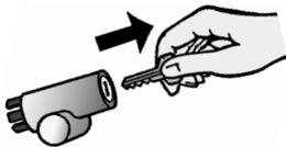
Before beginning, turn off the ignition and remove the ignition key. If necessary, remove the main circuit switch.
