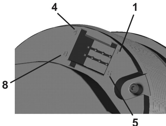
Depending on the configuration, insert the cable into the 8-pin contact enclosure according to the following pin assignment. The contacts must audibly lock into place.
