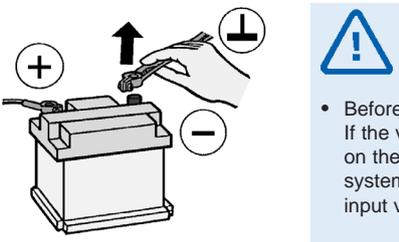
Disconnect the negative terminal on the battery. Make sure the battery cannot unintentionally restart.
