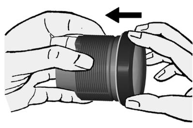
Place the new front ring on the instrument and press it on until it is flush with the instrument glass.
