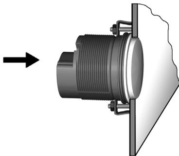
Place the flush mount seal A2C53215640 on the instrument glass. Put the instrument into the drill hole from the back. Adjust the instrument so that the gauge is level and fasten it to the stud bolts on the rear side of the panel, using the flush mount fixing bracket A2C59510864.
