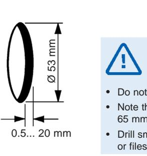
Conventional assembly. (Instrument is put into the drill hole from the front).
